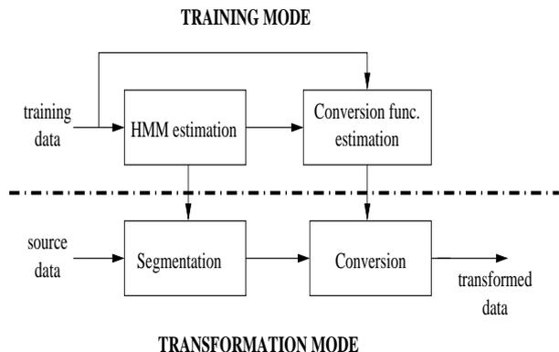
Figure 2: HMM-based VC system block diagram
