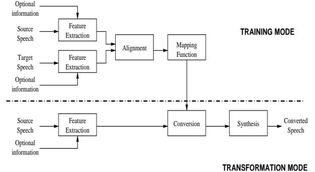
Figure 1: VC system block diagram
